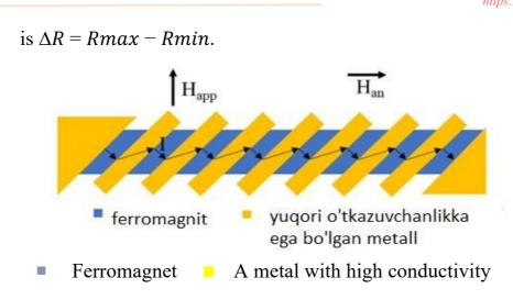
If this structure has a total magnetic anisotropy field, Han, and an applied external field, Happ, the resistance is given by [2]
