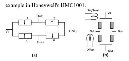
a) Magnetic resistance of AMR sensor together with Wheatstone bridge b) Construction of AMR sensor together with offset and set/reset panels
